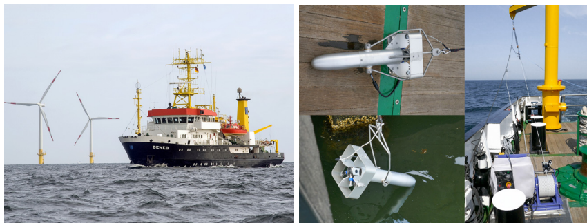
Fig. 1: The BSH survey vessel VWFS Deneb (left) and the newly installed (June 2020) AML Oceanographic MVP-30 underway profiling system (right)
