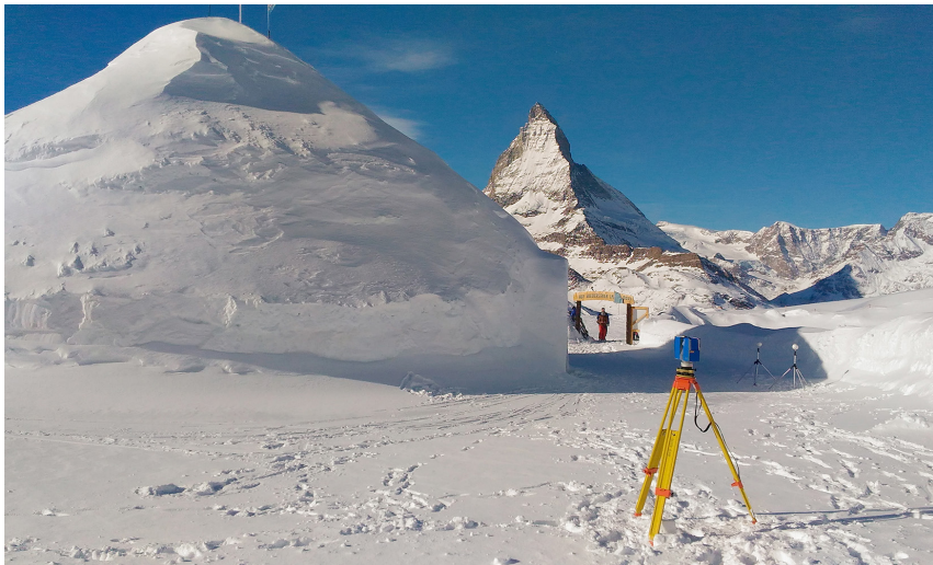
Fig. 1: The igloo, covered with non-compacted snow on the outside (laser scanner during an outside scan, two wooden spheres used for registration).
