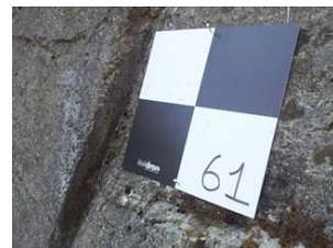
Fig. 4: Marker near a joint
