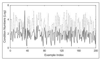
Fig. 3: Logarithmic condition numbers of matrices after applying the inverse integer Cholesky decorrelation. Solid line – iterated, dotted line – uniterated.
