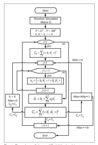
Fig. 4: Flow chart of the modified LLL algorithm.
