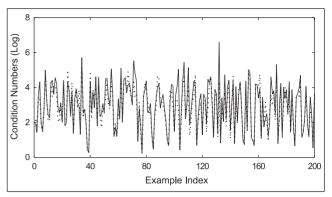
Fig. 5: Logarithmic condition numbers of matrices after applying the LLL algorithm. Solid line – iterated LLL algorithm, dotted line – uniterated LLL algorithm.
