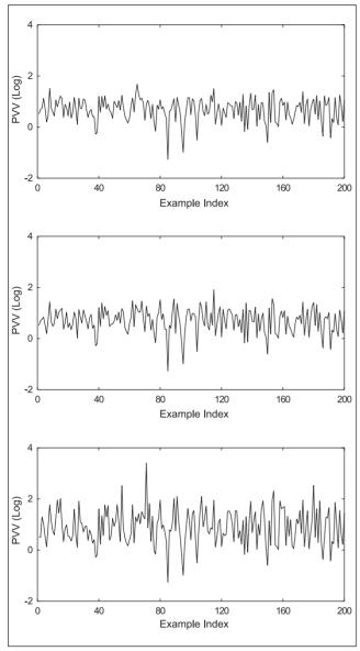
Fig. 16: Logarithmic value of  $log\{(z-z_0)^TQ_z^{-1}(z-z_0)\}$  after applying decorrelation: Upper plot – CHOL; Center plot – LLL; Lower plot – GAUS
