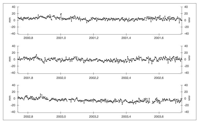
Fig. 2: Daily height differences between METS and MAR6 relative to the mean 19.1774 m during the analysed three years period
