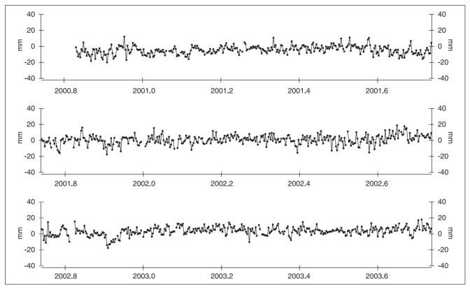
Fig. 4: Daily height differences between VILØ and TRDS relative to the mean 132.2774 m during the analysed three years period
