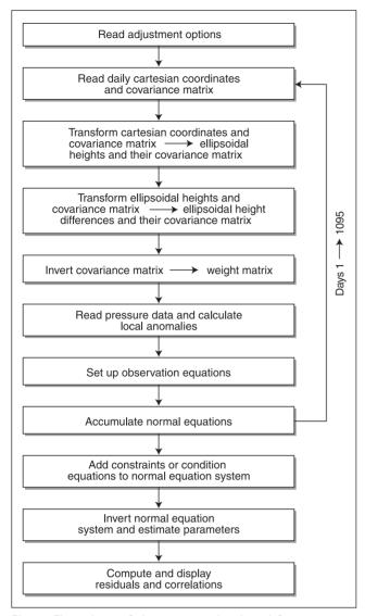
Fig. 5: Flow chart of the program developed for estimating uplift rates
