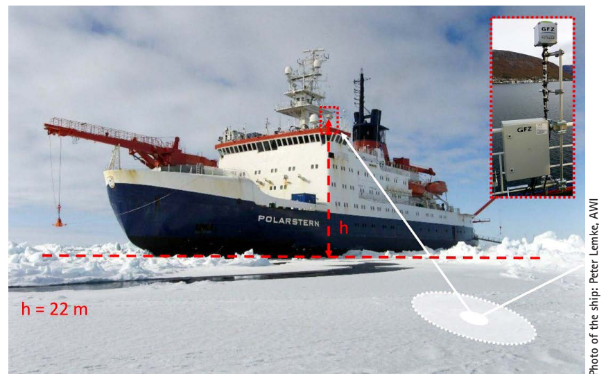
Fig. 16: GNSS reflectometry concept for sea ice observations using the GFZ setup aboard R/V Polarstern .
