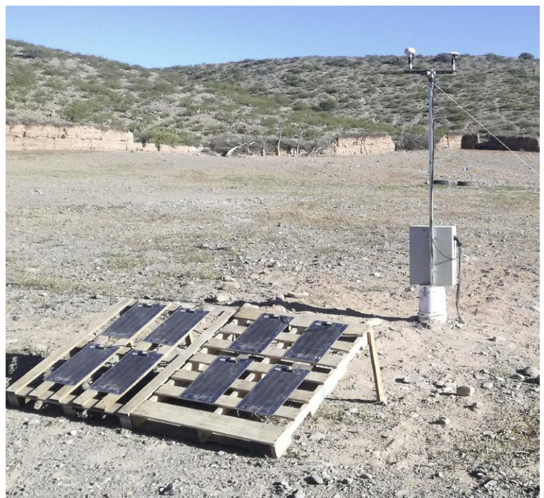
Fig. 21: GNSS station installed in Payogasta, Salta, Argentina. The station is powered by solar panels and it is equipped with a Novatel SMART-V1G and a Geostar GeoS-5M EVK GNSS receiver.
